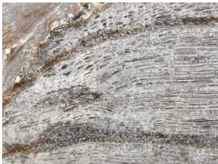
Fig. 9: Detail from Fig. 8, interfascicular rays, W approx. 3 mm
